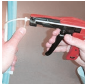
Grip the cable tie with the tool.
